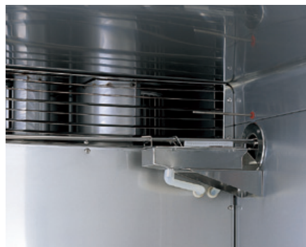
Wick installation (Test area)
